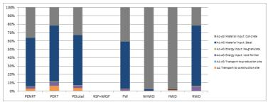
The impact indicators are also significantly influenced by the production process associated with the base materials concrete and steel (90-97%). In the case of ODP, POCP and ADPF in particular, the steel component is dominant for flexural reinforcement and hollow reinforcement cages.
